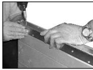
2. Fit door handle to the door. Place handle vertically onto door approx. 20mm from the edge of the door. Secure into place using 4x 25mm black screws.
